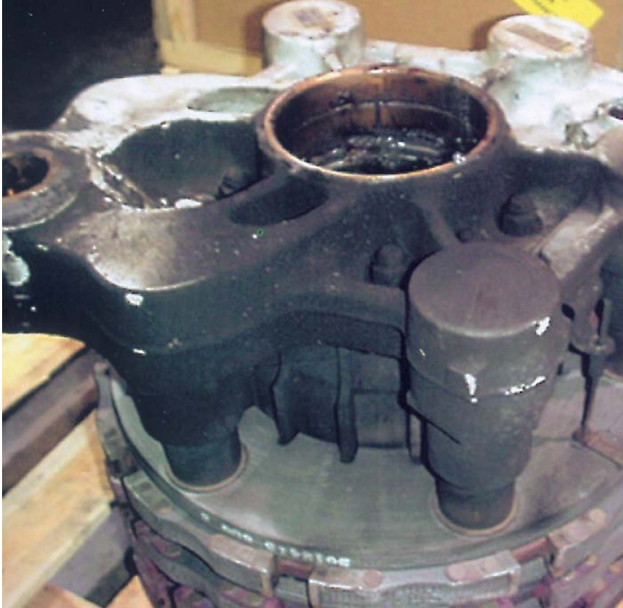
Figure 3: Removed brake following fire from hydraulic fluid leak
